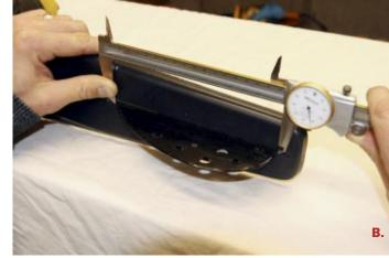
Fin Depth (A) is the point on the fin that is furthest away from the bottom of the ski. Since this is the easiest, most repeatable measurement you can take, I recommend it perpendicular to the bottom of the ski be your first.
